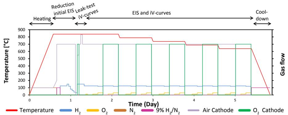
**Figure 1:** Test profile 'fingerprint', SOFC stack or single cell testing with characterization by iV and EIS.
