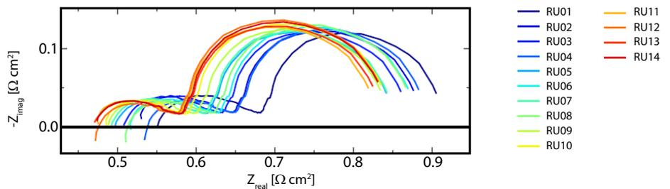
**Figure 2:** Simultaneous electrochemical impedance spectroscopy (EIS) on a 14 cell stack (repeating units). It shows relatively identical EIS shapes, but displacement of results (series resistance) is due to thermal gradient across the stack. Recorded at 700 °C, fuel: 20 % H<sub>2</sub>O and 80 % H<sub>2</sub>, oxidant: Air [1].
